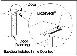
appropriate adhesive either in a channel or flush to the surface. BlazeSeal™ may be supplied with a factory applied pressure sensitive adhesive film.
